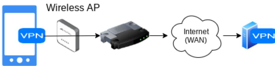
Figure 2: Client connects to VPN endpoint via foreign AP
